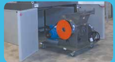
Step 3: Replace knives and perform other maintenance with easy access.
