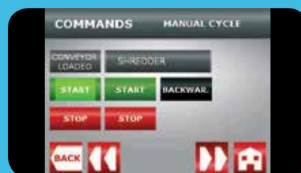
Single button integrated controls for activation of associated loading, conveying, refining, and discharge systems.
